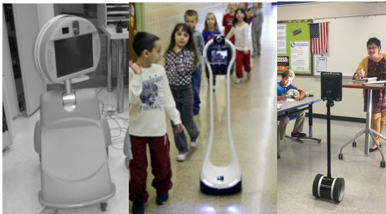
Figure 5.1. Three telepresence robots in school. Left to right are PEBBLES, VGo, and Double.
