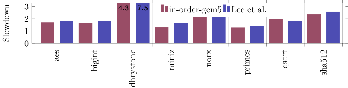
Figure 6.2: Comparison of slowdowns (incurred by trusted execution using Keystone) between gem5 and Lee et al. [1]. This slowdown includes enclave creation and management time as well.
