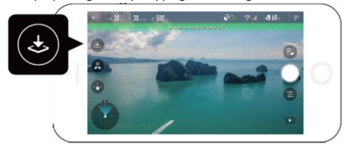
2. Manipulate the YI Pixie drone to the environment available for safe landing, and click the "One-key return" icon on the APP control interface, following which the YI Pixie drone will slowly go down to the ground.
