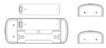
Red indicator normally on: The battery voltage is lower than 4.2V
