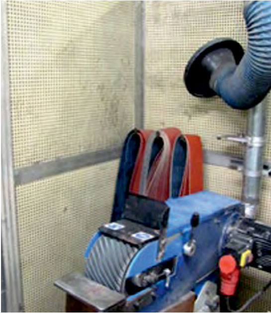
Figure 13 Movable acoustic screen in a foundry
