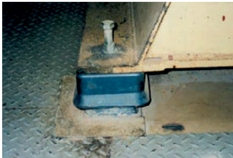
Figure 7 Detail of vibration-isolating mount
