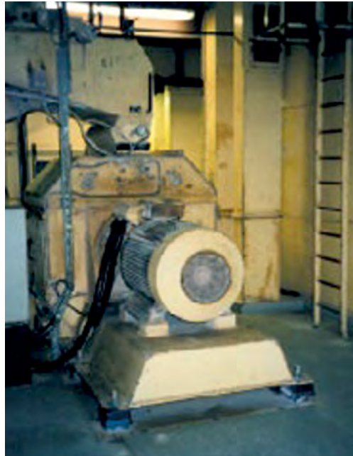
Figure 6 Vibration-isolating mounts reduce vibration entering the floor
