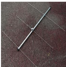
(a) VHF Yagi antenna
