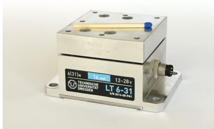
Fig. 7 Redesigned moving-magnet linear table: travel range 14 mm, nominal/peak force \pm 6/\pm 31 N, integrated absolute position sensor with 0.16 \mu\text{m} resolution, integrated control electronics with CAN hardware for implementation of CAN interface
