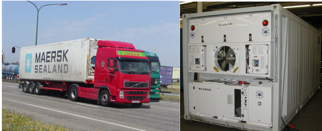
Figure 1-1: Truck with refrigerated cargo container (source: Wikimedia Commons 1 ) and Klunge Corporation Redundant Refrigeration System (source: Wikimedia 2 )
