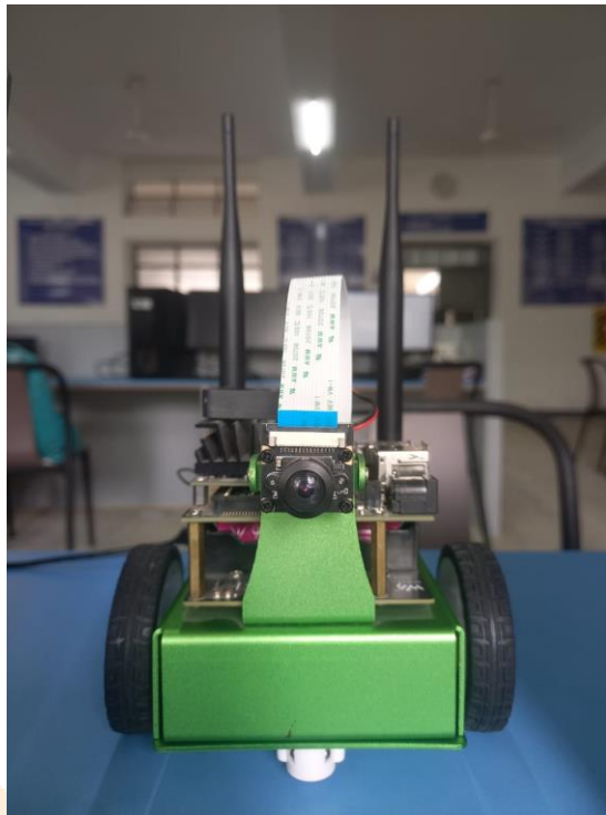
Fig.3: JetBot Hardware and Final Bot.
