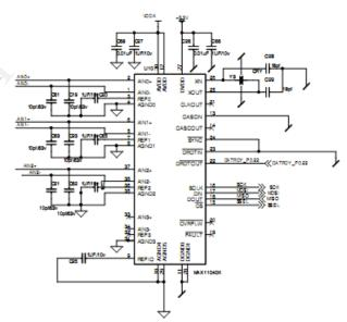
Here the system uses MAX11040K is 24 bits, four channels, simultaneous-sampling, sigmadelta analog-to-digital converters (ADCs) from MAXIM manufacturer. ADC s has four modulators simultaneously convert each fully differential analog input with a programmable data output rate ranging from 0.25ksps to 64ksps. The devices achieve 106dB SNR at 16ksps and 117dB. SNR at 1ksps (MAX11040K). The differential analog input range is ±2.2V.
