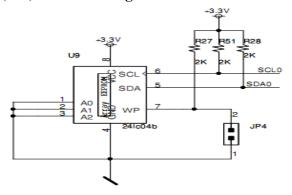
Low-voltage design permits operation down to 1.8V, with standby and active currents of only  $1~\mu A$  and 1mA, respectively. The 24LC04B also has a page write capability for up to 16 bytes of data. It is for the purpose of storing saved data file names.
