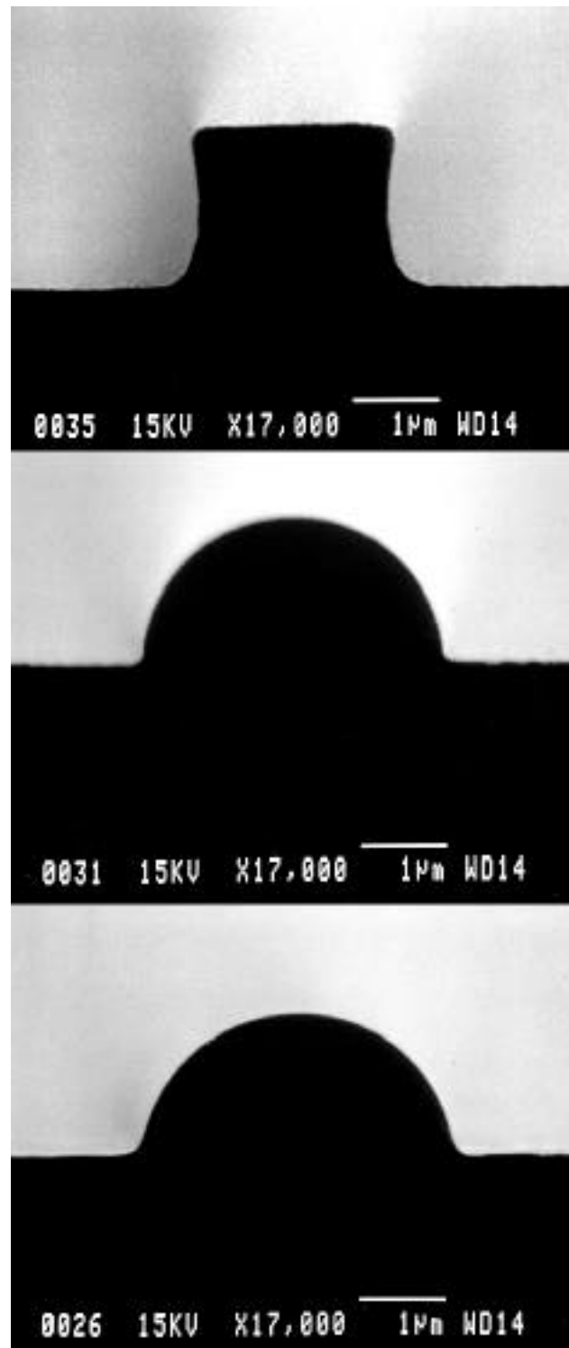
Figure 5 Cross-sectional SEM of a 6 micron wide stripe of positive resist and the same stripe after 2 minutes and 4 minutes of exposure to a hot plate at 125C. Both photoresist patterns are supported by a 2 micron filter/focus layer of dyed photoresist.
