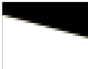
Figure 5. When we reproject an orthoimage to a different UTM zone, empty wedges appear again (right). The borders of these wedges have “intermediate” values due to resampling
