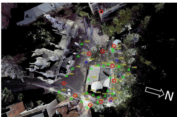
Figure 4. Overview of the registered Faro total point cloud with distribution of positions (red) and target marks (paper marks green, profit targets blue)
