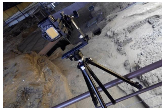
Figure 3. Image data acquisition with Nikon D80 for the generation of the virtual tour.
