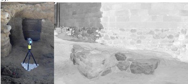
Figure 8. Data acquisition with the Faro-Focus3D 120 (Left) and the corresponding range image obtained (Right).
