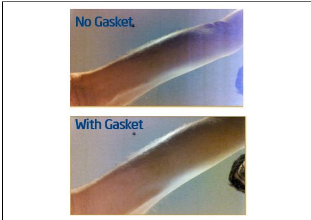
Figure 7-15. Example of Light Leakage Effects
