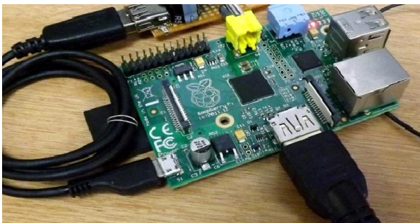
Fig-7.4 Raspberry pi connected with UART
