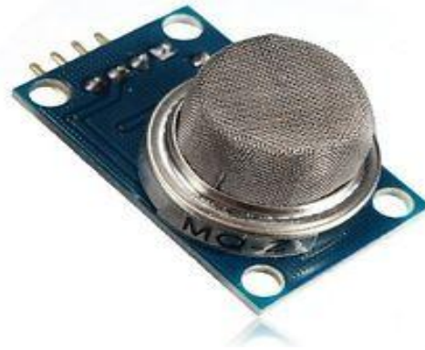
Fig-5.1.1: Mq2 arduino gas sensor
