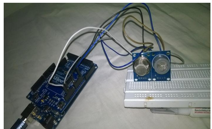
Fig-7.2: Interfacing sensors with arduino
