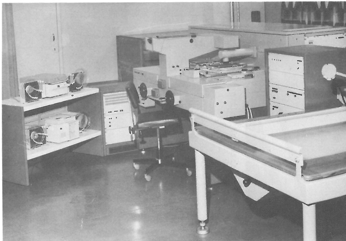
Fig. 1 Topocart with Orthophot D 300, electrical cabinet, Digital Control Unit, punched tape periphery, and drawing table
