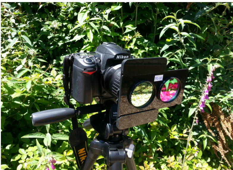
Image 2: A UV camera setup with our custom-built filter slider that makes it easy to take the same photo in visible or UV bands.
