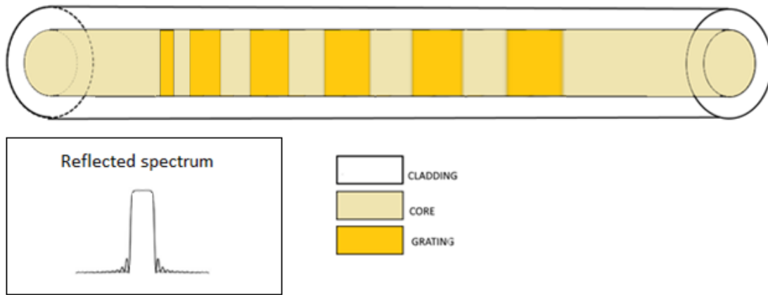
Figure 7. Chirped FBG. Inset: reflected spectrum.
