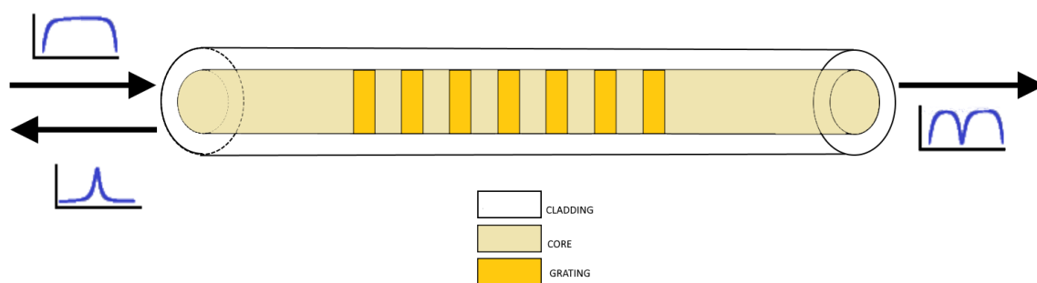
Figure 4. FBG index profile. In insets, the spectrum of the incident, reflected and transmitted beams.
