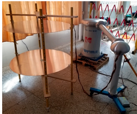
Figure 18. Power frequency voltage division ratio calibration platform.
