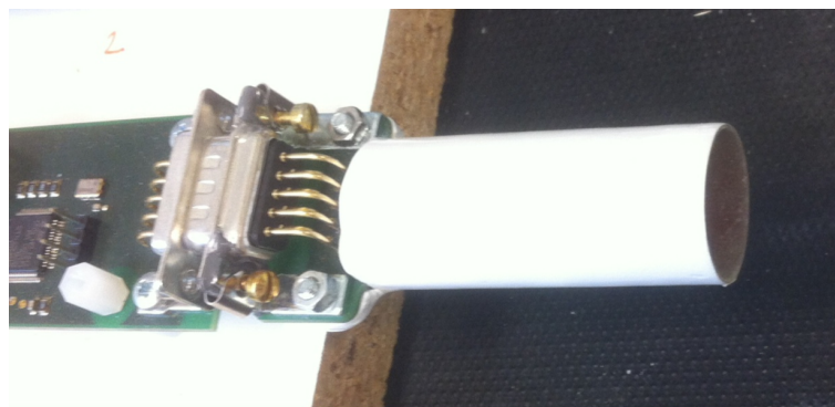
Figure 2. Sensor nozzle for a well-defined environment (total pressure conditions with a well-defined flow rate) for a fine wire temperature sensor. Inside the tube (not visible), the PCB (printed circuit board) to execute raw measurements and carry sensors is installed.
