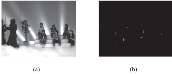
Fig. 1. (a) Texture image of Kendo sequence (view 3); (b) thresholding result using Otsu's algorithm (black: spatial-invariant regions, white: spatial-variant regions).
