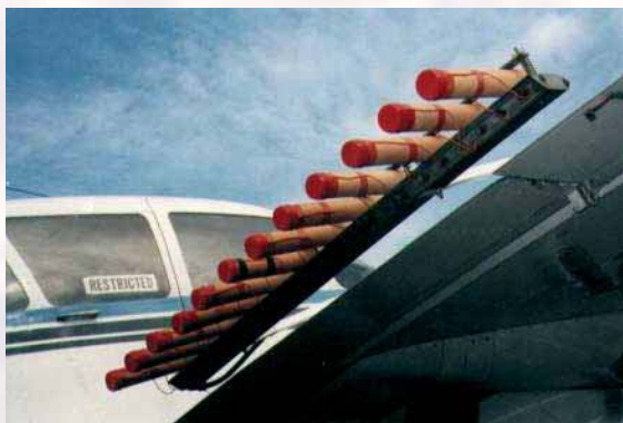
A cloud-seeding aircraft is equipped with sprays along both wings.
