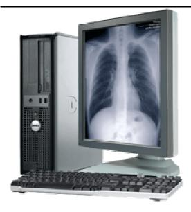
Vision Tools RadView is a very powerful and scalable acquisition and viewing station for CR/DR machines The RadView station can be connected to any DICOM compatible CR or DR machine.
