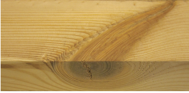
Figure 1. Grain behavior around a knot.
