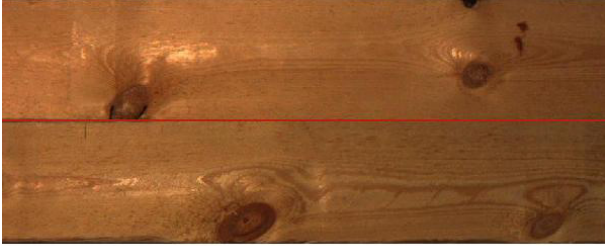
Figure 1. Grain behavior around a knot.
