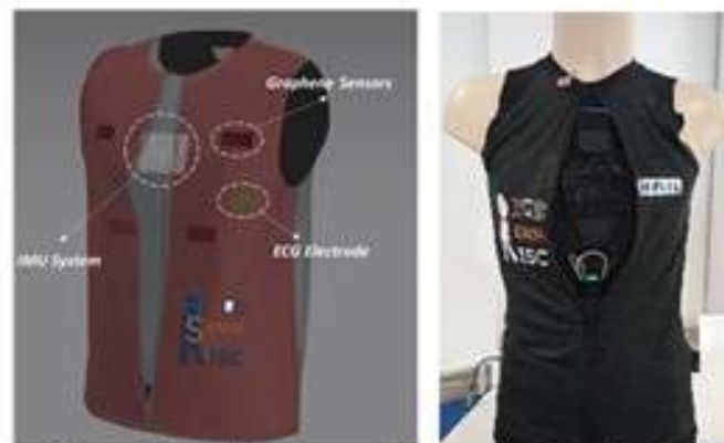
Figure 1 - wearable t-shirt with Bluetooth systems for physiological monitoring
