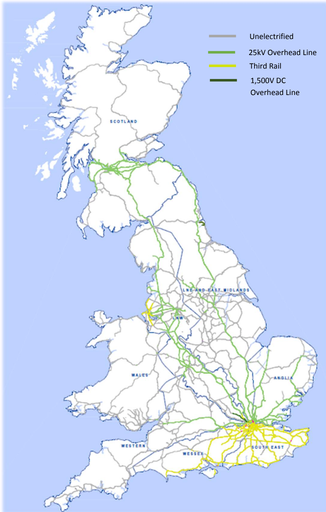
Figure 4: UK Rail network showing 25kV electrification in green and 750V DC third rail in yellow
