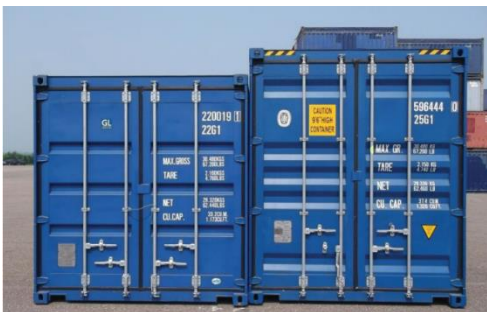
An example of the varying dimensions of different types of intermodal unit, with the larger 'high cube' varieties more challenging to accommodate on gauge constrained rail routes. Source: cratexcontainer.com
