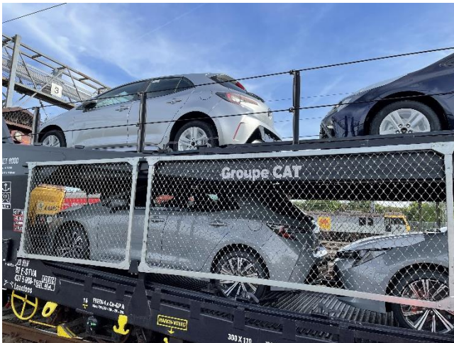
Refurbished car-carrying wagons. An enclosed top deck would help protect the valuable cargo, but would mean a larger wagon and therefore a gauging challenge Source: Network Rail
