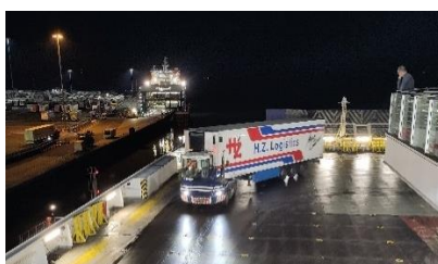
Unaccompanied ro-ro: semi-trailer being unloaded from a ferry by a tug vehicle
