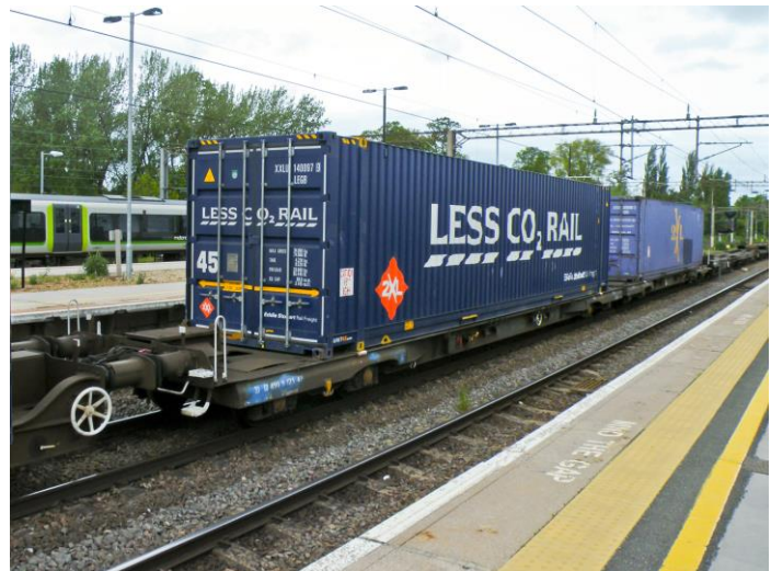
IKA megafret wagons have platforms that are lower to the track. These wagons are used to carry 'high cube' boxes, including wider refrigerated units, on the W9a gauge cleared network, where width clearance, but not height, has been achieved. Source: Dan Adkins
