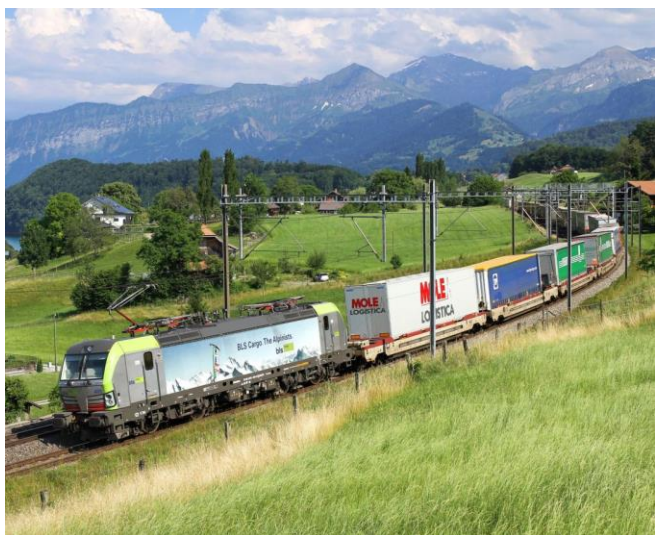
A piggyback intermodal service carrying unaccompanied semi-trailers Source: www.cargobeamer.com
