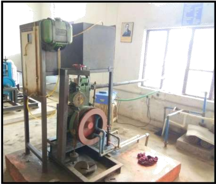
Fig 4.2: Four Stroke, Single Cylinder, Vertical Diesel Engine
