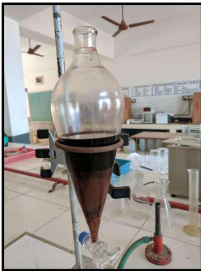
Fig 3.2: Separation of Glycerol and Esters
