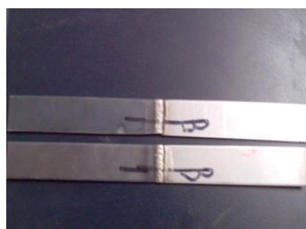
Fig-5, Test specimens for bend tests
