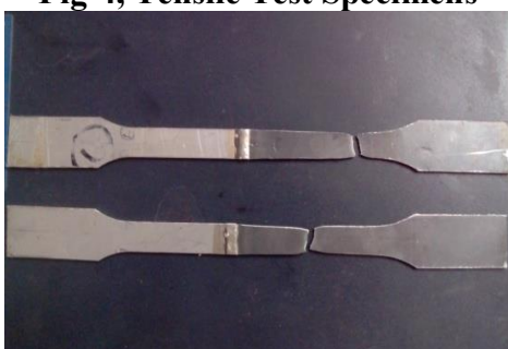
Figure-6, Test Specimens showing failure at CS side away from weld and HAZ
