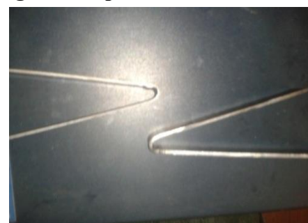
Figure-7, Test Specimens showing satisfactory weld properties
