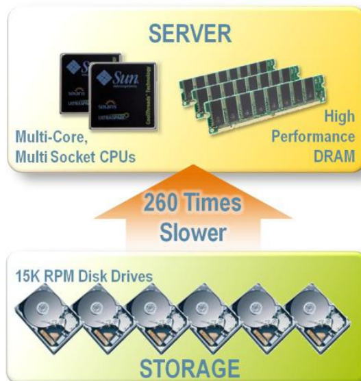
Figure 1: Even the fastest HDDs are much slower than today's CPUs and can hold back application performance.
