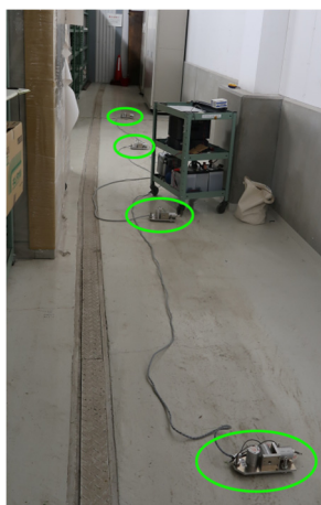
Figure 16: Sensors for wave velocity measurement.
