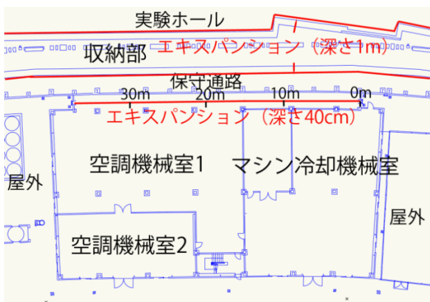
Figure 3: View of machine room and expansions.
