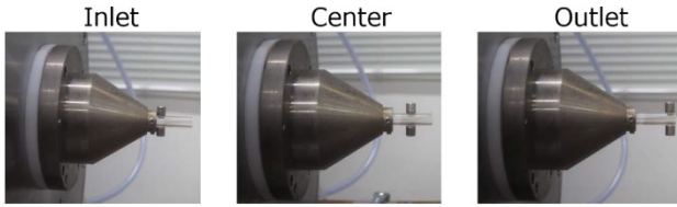
Figure 3: Inner electrodes of the PFD.
