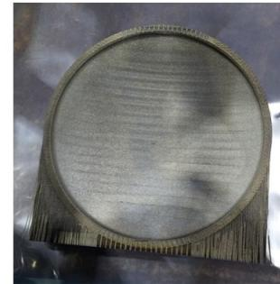
Figure 4: Pictures of the sphere window with a diameter of 60 mm and with a thickness of 0.2 mm (UP) and the window with a diameter of 166 mm and with a thickness of 0.6 mm (DOWN).
