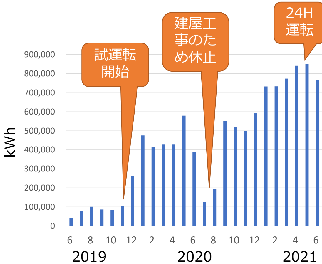
Figure 3: Monthly consumed electric power in the SAGA-HIMAT facility.
