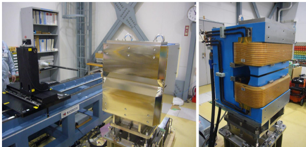
Figure 6: Photographs of the DC septum with septum and magnetic shield (left) and without the shield (right).
