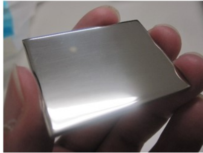
Figure 7: Sample of the metal window manufactured by only machining.
