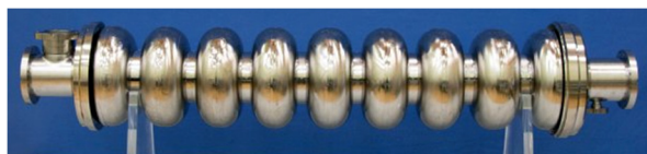
Figure 1: 1.3 GHz SRF cavity made by LG niobium (KEK-2) [1].
