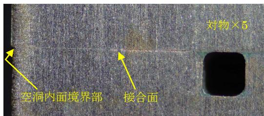
Figure 6: Cross-section of the test piece after brazing.
