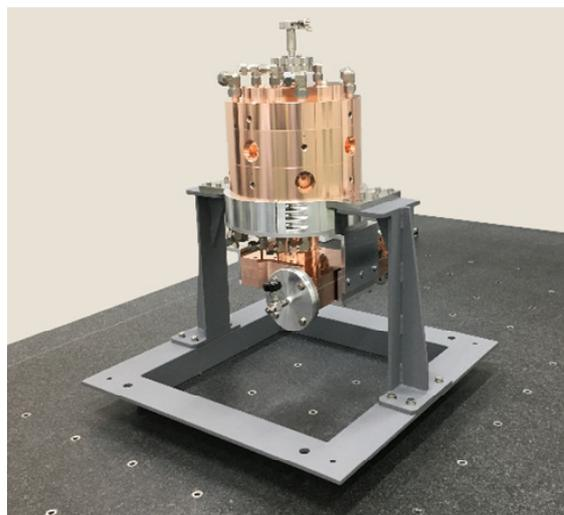
Figure 7: SCPC after brazing and dimple tuning.
