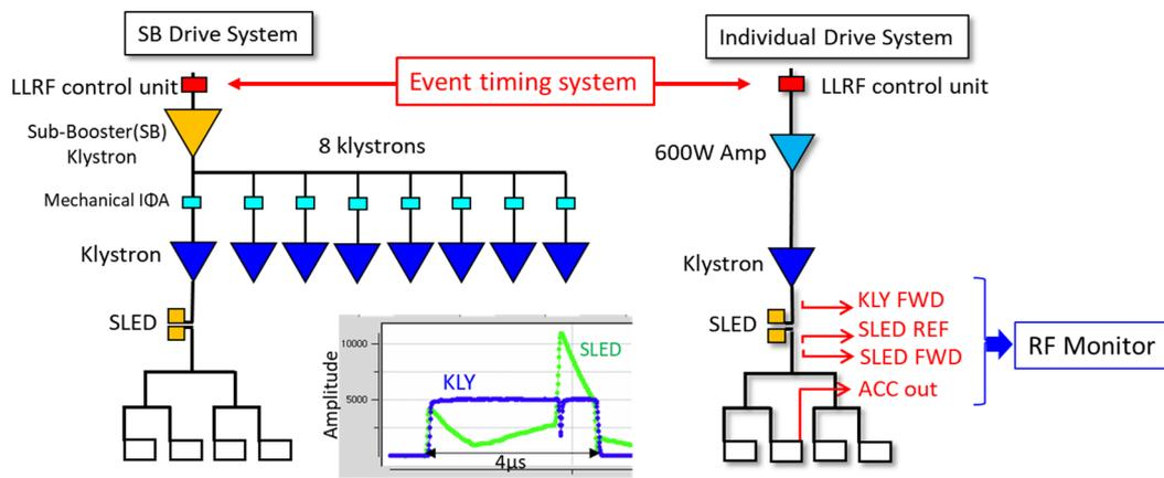
Figure 1: RF drive system at the KEK e<sup>-</sup>/e<sup>+</sup> injector LINAC.
