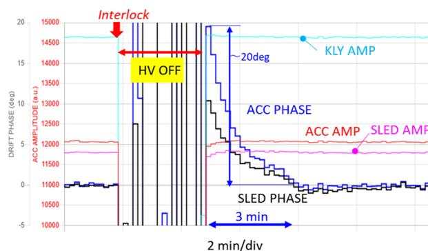
Figure 4: Amplitude and phase after HV down.
