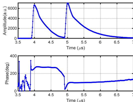
Figure 3: Reflection wave form of the RF gun.
