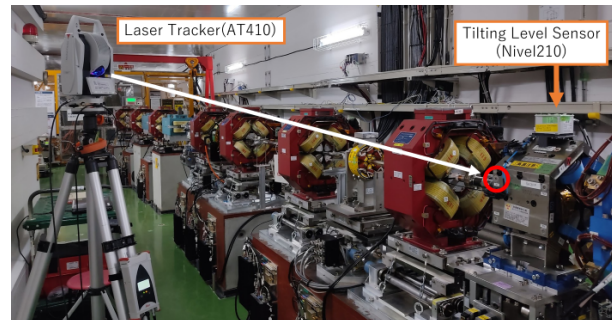
Figure 9: Positioning measurement with Laser Tracker (LT). Red circle: LT measurement point.
