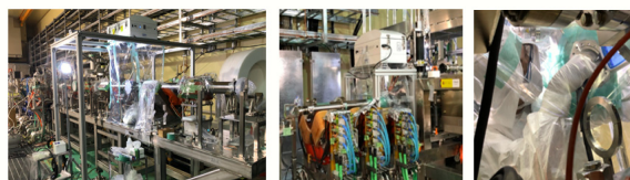
Figure 5: MEL assembly in clean environment.
