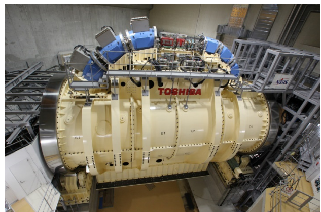
Figure 2: Photo of the superconducting rotating gantry in new particle therapy facility.
