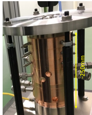
Figure 2: Laser-driven photocathode electron gun.
