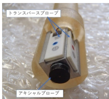
Figure 6: Assembling Hall elements.
