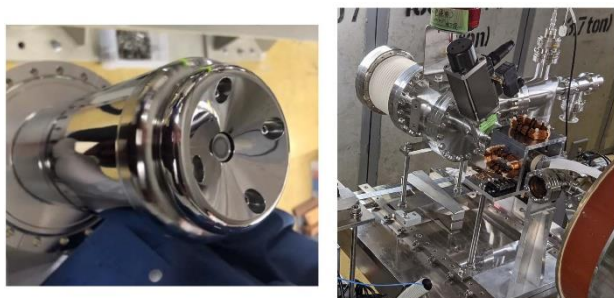
Figure 2: Pictures of the cathode part (Left) and the thermionic electron gun (Right).
