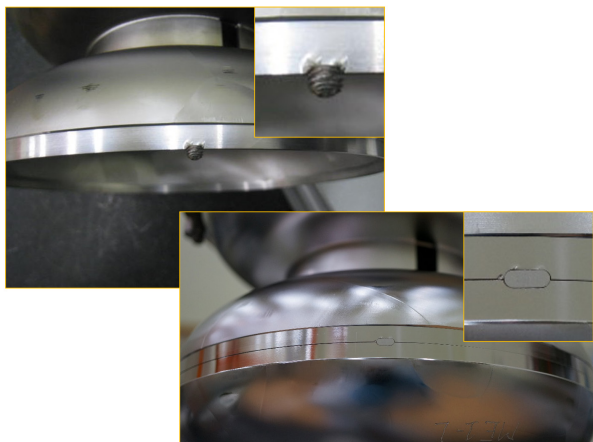
Figure 7: The dumbbell that a set screw bit on the equator. The left picture shows the set screw attached on the equator, and the right picture shows the small niobium tip embedded in the repair point before welding.
