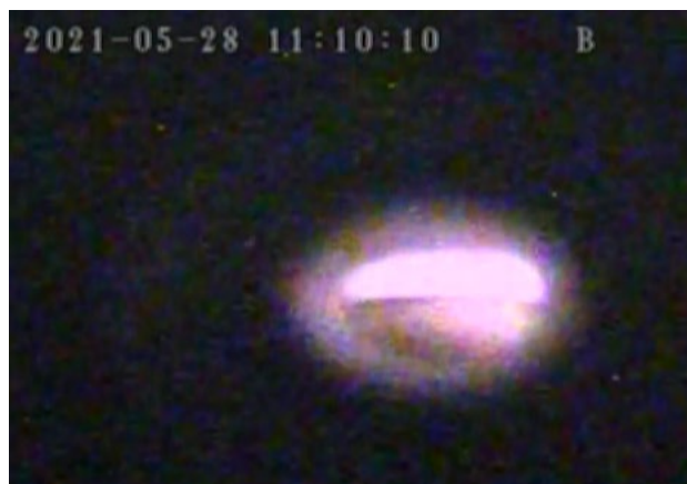
Figure 4: Example of images of light emitted from the RF window recorded with the high-sensitivity camera ( P_{\text{inp}} = 218 \text{ kW} ).
