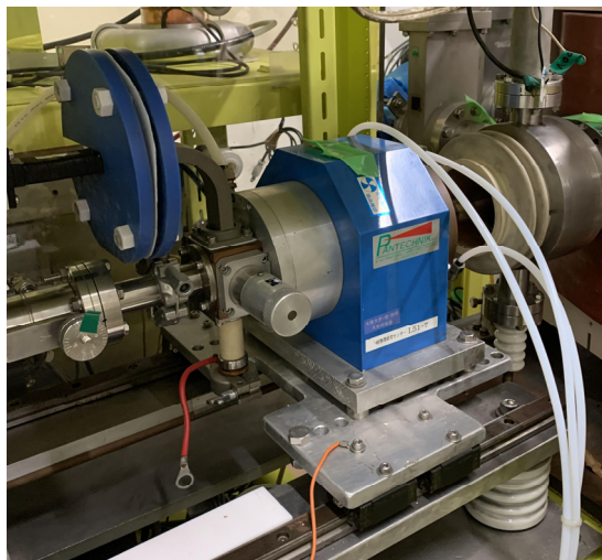
Figure 2: The 10GHz permanent magnet ECR NANOGAN (PANTECHNIK): It has two extraction electrodes. It is possible to apply 15 kV between these electrodes, and it is also possible to apply 35 kV between first extraction electrode and plasma electrode.
