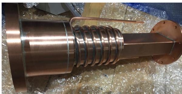
Figure 4: Plasma chamber used for test bench.
