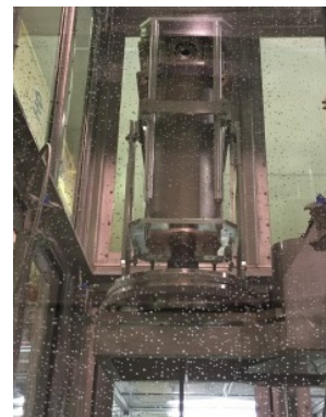
Figure 4: High-pressure rinse for RIKEN-QWR.
